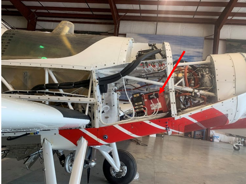
Figure 3 (T-34 Battery Disconnect Shown)
